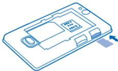
★ **Tip:** To remove the memory card, push it in until it's released, then pull it out.
