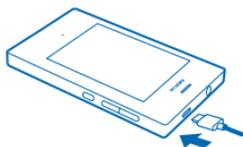
If the battery is completely discharged, it may take several minutes before the charging indicator is displayed or before any calls can be made.
