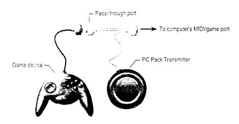
Always turn your computer off before you connect or disconnect the Transmitter to or from the MIDI/game port on your computer, or before you connect or disconnect a game device to or from the Transmitter's Passthrough port.
