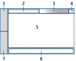
The touch screen consists of the task navigator (1), the application title area (2), the status indicator area (3), the minimize and close buttons (4), the application area (5), the toolbar (6), and the application switcher (7).
