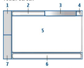
The touch screen consists of the task navigator (1), the application title area (2), the status indicator area (3), the minimize and close buttons (4), the application area (5), the toolbar (6), and the application switcher (7).
