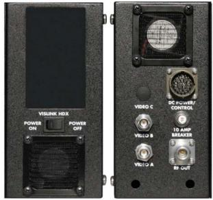
The amplifier operates at 8W for all bands except 4940-4990 MHz which is limited to 1.0W maximum. Low power mode is typically 3 to 6 dB below the maximum rating.
