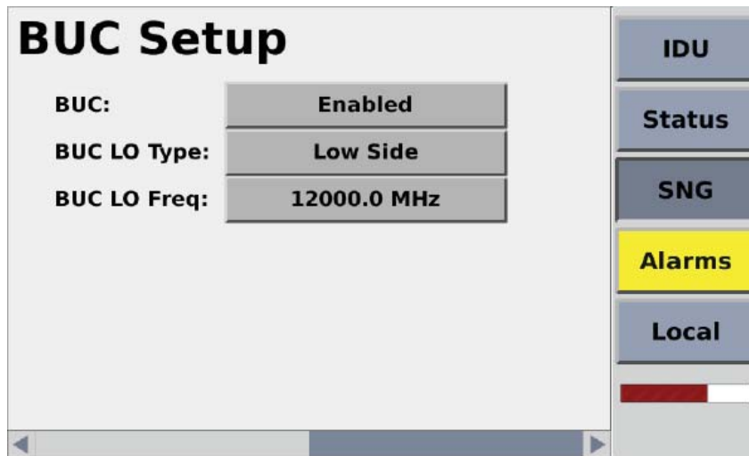
Figure 26: NewStream SNG Touchscreen - BUC Setup Frequency Tune Mode
