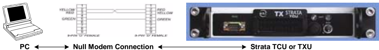
Figure 5 – Serial Data Connection Details
