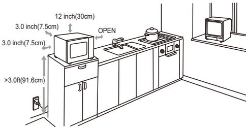
A minimum clearance of 3.0 inches (7.5cm) is required between the oven and any adjacent walls. One side must be open. The minimum installation height is 3.0ft(91.6cm).
