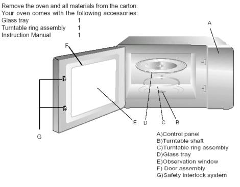
Shuts off oven power if door is opened during operation.
