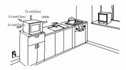
A minimum clearance of 3.0 inch (7.5cm) is required between the oven and any adjacent wall. One side must be open.
