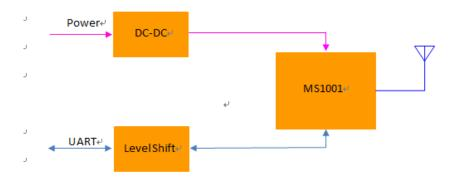
figure 1. Module System Block Diagram
