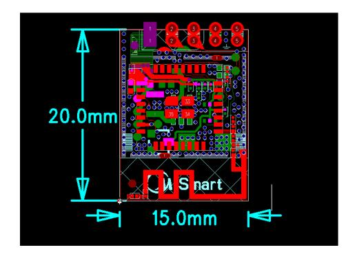
The size of the module as shown above, length 20mm, width 15mm, thickness 1.0mm (error +/- 0.1mm)
