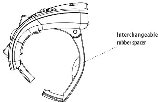
In the box you will find two extra rubber spacers to be replaced in case your handle has a different size
