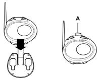
BT SKI is maintained in position thanks to the fixing clip located on the upper section (A).
