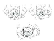
In case you have a rigid helmet, you should mount your BT SKI system by using the biadhesive plate.
