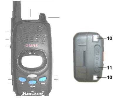
1-Up/Down Buttons 2-Monitor Button 3-Push to Talk Button 5-Call Button 6-Accessory jacks 7-On/Off Volume Control 8-Enter Button 9-Function Button 10-charging contacts 11-Charge Jack
