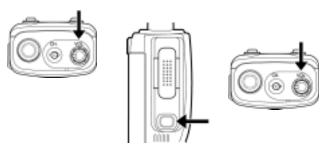
Use the channel switch to choose the desired channel.
