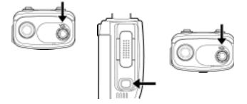
To transmit, place the radio microphone approximately 1.5" from your mouth then press and hold the P-T-T bar while speaking in a normal tone. Release the P-T-T bar when you are finished speaking; the radio will be placed into receive mode.
