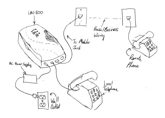
The longest length of cabling for which the SAU-1900E has been designed is 1000 feet (305 meters). This should be sufficient for most installations. However, if your wiring is longer than 1000 feet, you may experience some audio problems with your telephone(s).
