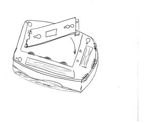
4. Line the holes in the bottom part of the bracket with the holes in the SAU-1900E.
