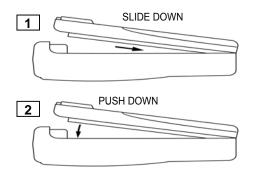
Hold the transceiver's body with one hand and the battery pack with the other. Put the battery pack onto the bottom of the transceiver.
