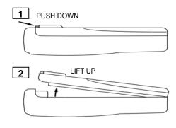
Press the battery release button located in the back of the battery pack.
