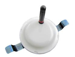
Badge signals received by VER-4452 RF Sensors are used to notify the Versus system of badge button presses, Remote Station button presses and badge battery status. RF also acts in a supervisory capacity, prompting the system to continue to display the last known IR location of badges that are not currently being detected by IR sensors.
