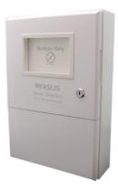
An internal IR XL Sensor reads the IDs of badges inserted through a slot on the front of the unit and sends real-time updates to the system. When used in combination with specific business rules, the Badge Drop Box automates many aspects of the patient visit cycle, including removal of patient badge assignments at the conclusion of the visit, automated discharge messages and logging clinical actions and processes.
