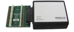
A punch-down connector block is included with each Collector. The connector block plugs directly into the 50-pin Amphenol connector on the side of the Collector. Up to four Collectors may be connected to any Concentrator; the Concentrator Plus (VER-2037) includes an internal Collector, so it can support up to three additional external Collectors connected in a daisy-chain fashion.
