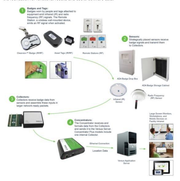
V-Direct sensory network components are easily identifiable by their physical characteristics and colors, but their part numbers provide important information about their functionality and compatibility. V-Direct IR Sensors with green or blue LEDs are XL Sensors; non-XL Sensors either feature another LED color or lack an LED. All V-Direct Badge Storage Cabinets and Badge Drop Boxes incorporate XL Sensors. All V-Direct Sensors can be used on any V-Direct Collector/Concentrator chain.
