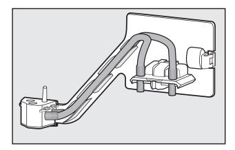
■ Remove the cover with the milk pipework. Clean the whole part in the dishwasher without taking it apart.
