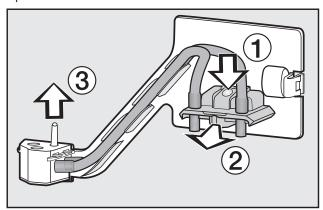
Do not pull the milk hoses off the retainers. This may cause the milk pipework to leak.
