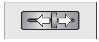
■ Push the slide control to the left for a finer grind or to the right for a coarser grind.
