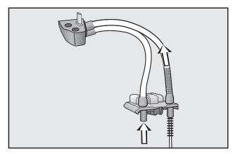
■ Insert the brush into the milk hoses one after the other from below. Push the brush back and forth to the end until there is no more no milk residue in the hoses.
