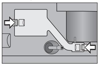
■ Unlock the cover for the milk pipework by pressing in the two brackets on the left and right.
