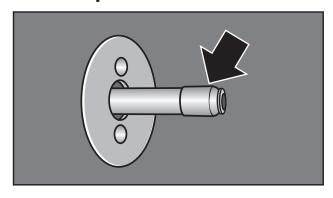
A connecting piece between the brew unit and the main dispenser is located on the inside of the door.
