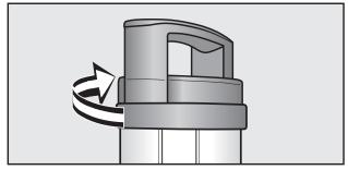
To rinse the pipework in the lid of the stainless-steel milk container, fill the large cleaning container to the "max." mark with **cold** water.
