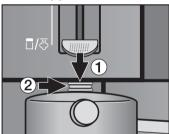
■ Press the steam lever, ①, down and "connect" the valve with the cappuccinatore, ②.
