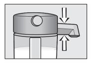
Press the spout together from the top and bottom to pull out the two pieces of the spout together. See below.
