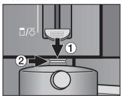
■ Press the steam lever, ①, down to connect the valve with the cappuccinatore, ②.
