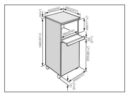
The display cabinet is intended to hold the CVA 2660 and an optional ESS 2060 Storage Drawer or EGW 2060 Cup Warmer.
