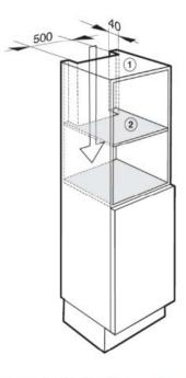
To ensure that the Combi Steam Oven has adequate ventilation, the following cut-outs measuring 19 11/16" x 19/16" ( $500 \times 40$  mm) must be made:
