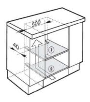
To ensure that the Combi Steam Oven has adequate ventilation, the following cut-outs measuring 19 11/16" x 1 9/16" (500 x 40 mm) must be made:
