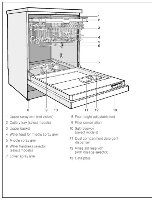
Figure 1-1: Appliance Overview - Typical Integrated Model
