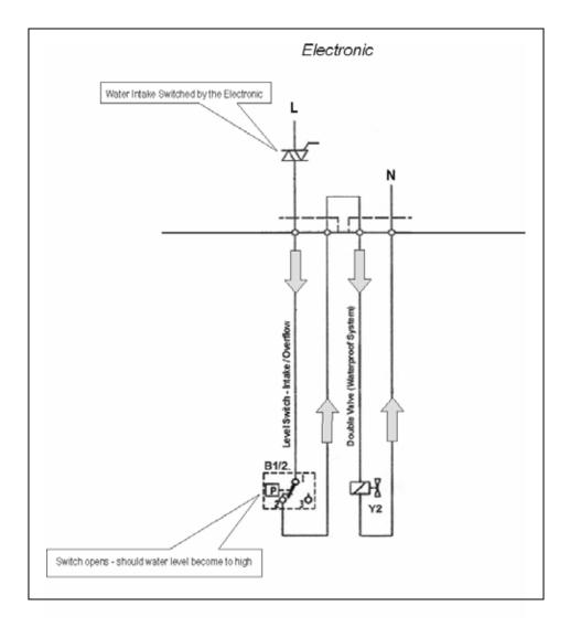
Figure 4-18: Water Intake / Level Switch Circuit
