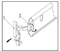
Figure 5-10: Stopper removal
