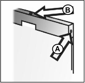
Figure 5-41: Removing the Fixing Bracket
