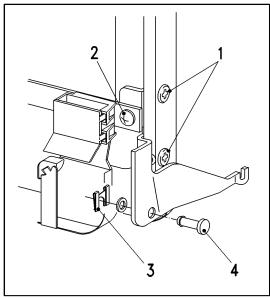
Figure 5-16: Hinge Removal
