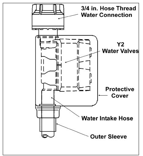
Figure 4-6: WaterProof System Connection
