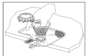
Figure 5-22: Pressing and Locking the Filter Assembly.
