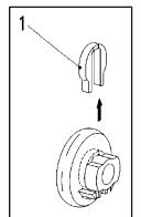
Figure 5-8: Bolt and Retaining Clip
