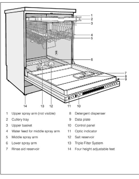
Figure 1-2: Appliance Overview – Typical Fully Integrated (Vi) Model
