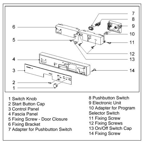
Figure 5-40: Control Panel (Novotronic and Touchtronic Dishwashers)
