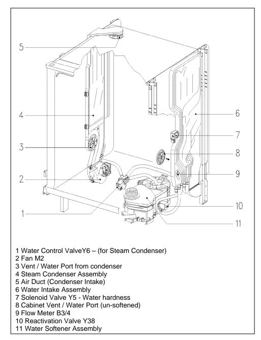
Figure 4-15: Components for the Condenser Drying System
