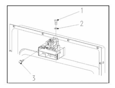
Figure 5-15: Lock Removal
