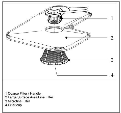
Figure 4-5: Filter Assembly
