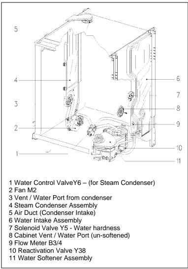
Figure 5-27: Steam Condenser Components
