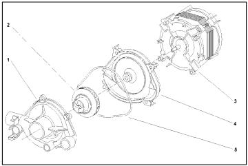
Figure 5-29: Components within the Circulation Pump
