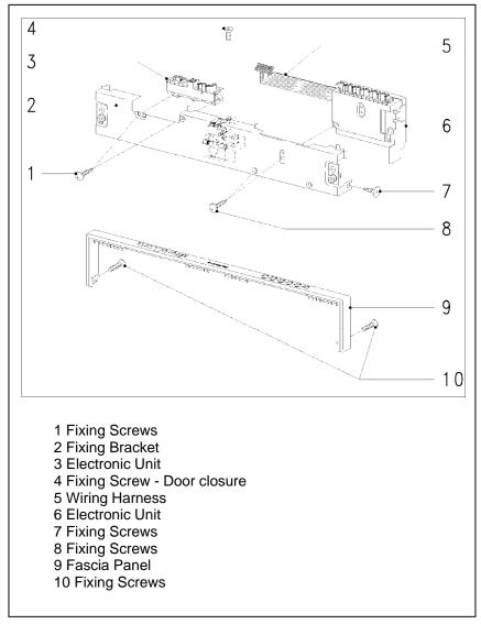
Figure 5-39: Fully Integrated (Vi) Control Panel
