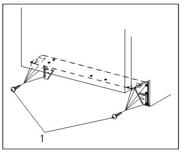
Figure 5-6: Plinth area with Connecting Strip
