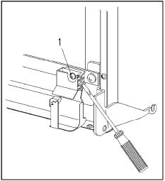
Figure 5-14: Cable Holder Removal
