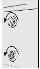
Figure 5-25: Water Inlet - Removal
