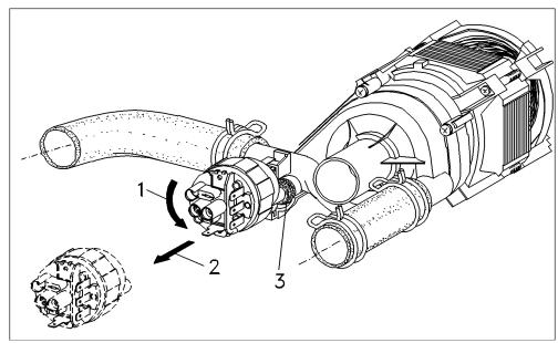
Figure 5-33: Heater Level Switch and Circulation Pump
