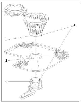
Figure 5- 21: Microfine Filter – Replacement
