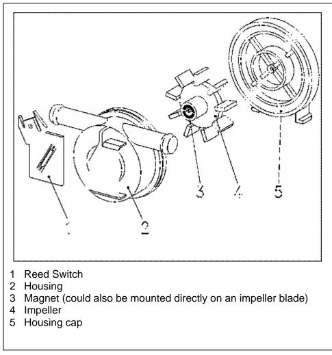
Figure 4-8: Flowmeter Assembly Components (External Flowmeter Shown)
