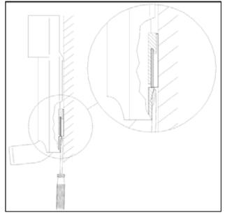
Figure 5-18: Middle Spray Arm Cover Removal
