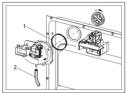
Figure 5-12: Fan Removal
