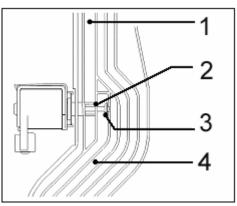
Figure 4-13: Water Hardness Mixer Solenoid
