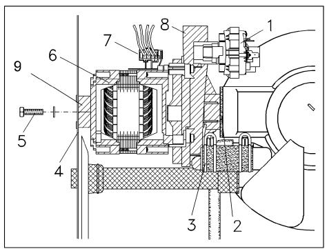
Figure 5-28: Circulation Pump – Removal
