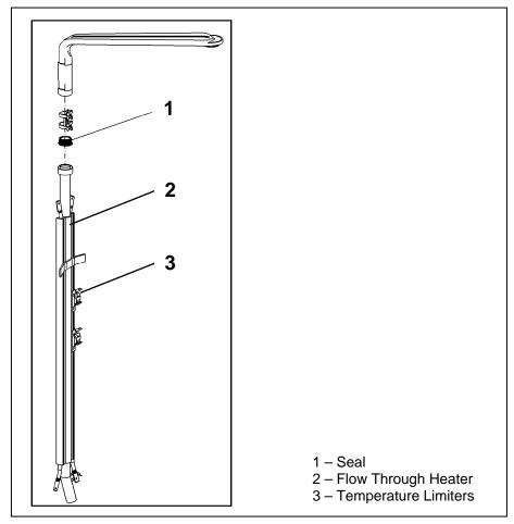
Figure 5-20: Flow-Through Heater with Seal (Item 1).
