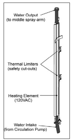
Figure 4-3: Flow Through Heater
