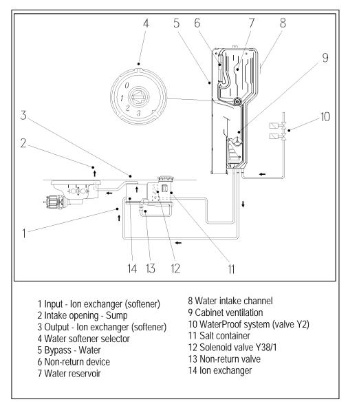
Figure 4-9: Water Intake System Equipped With Integrated Flowmeter
