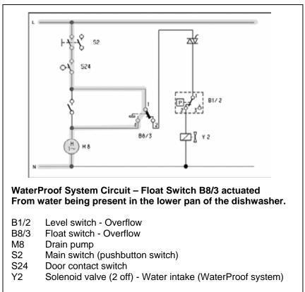
Figure 4-7: Water Intake Circuit
