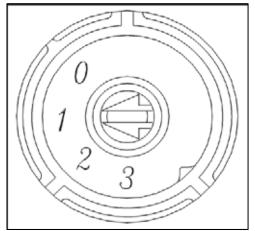
Figure 4-10: Water Hardness Selector
