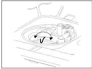
Figure 5-32: Turning the Circulation Pump Tool
