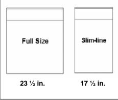
Figure 1-6: Dishwasher Widths
