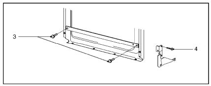
Figure 5-13: Inner Door Panel Removal
