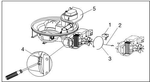
Figure 5-34: Drain Pump - Replacement
