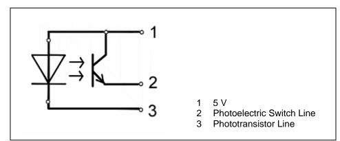
Figure 4-20: Turbidity Sensor (ECO Sensor)
