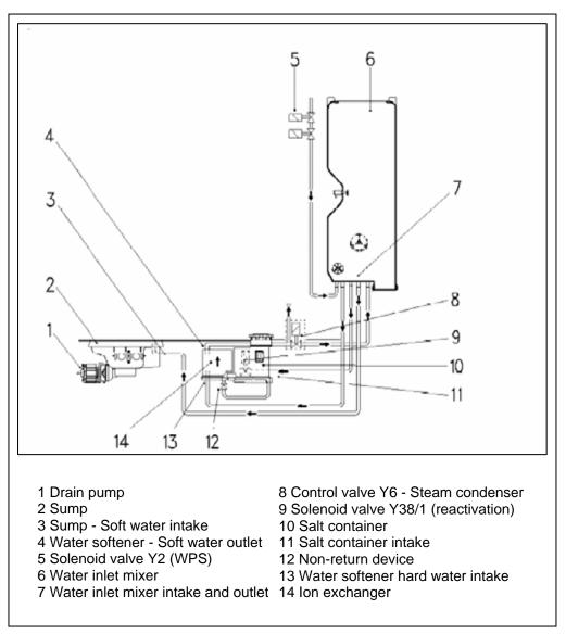
Figure 4-11: Water Path with Integrated Flowmeter
