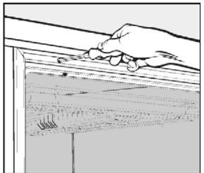
Figure 5-17: Door Tension Adjustment Screw
