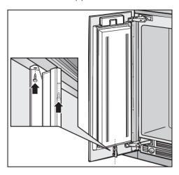
■ From below, screw the air separator firmly onto the door with the 2 screws.
