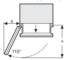
Miele recommends using the full door opening angle of 115° for this freezer.
