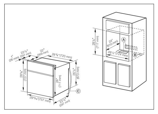
A Vent cut-out (min. 24"<sup>2</sup> / 150 cm<sup>2</sup>) possible at rear or platform of cabinet
