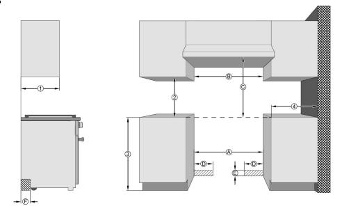
${}^{\hbox{$\footnotesize{\tiny \$}$}}$  In case of combustible construction, an additional minimum clearance of 6" (each side) is necessary.
