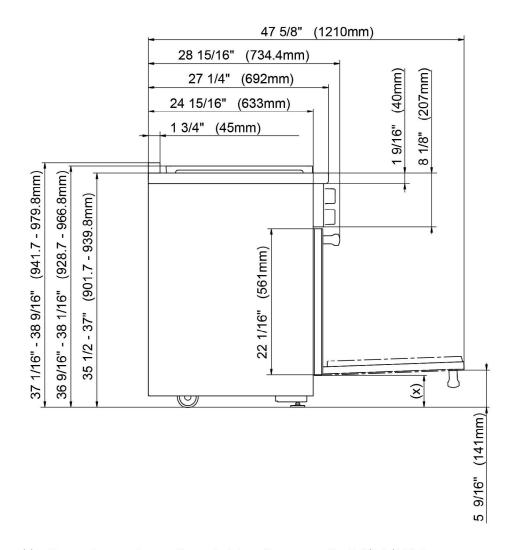
(x) = Depending on the appliance height adjustment:  $4" - 5 \frac{1}{2} " (101.6 \text{ mm} - 139.7 \text{ mm})$
