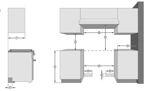
® In case of combustible construction, an additional minimum clearance of 6" (each side) is necessary.
