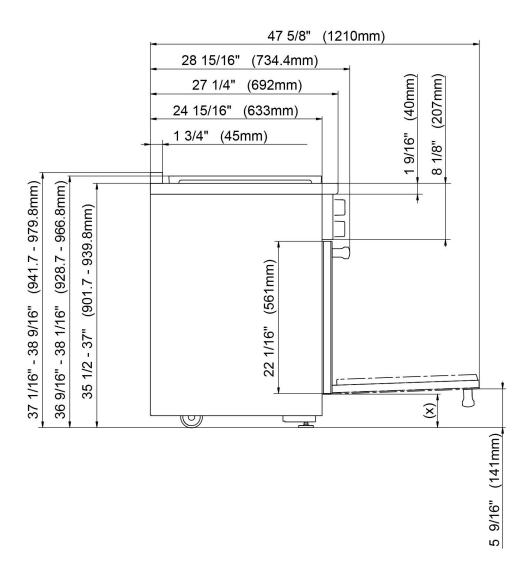
(x) = Depending on the appliance height adjustment:  $4" - 5 \frac{1}{2} " (101.6 \text{ mm} - 139.7 \text{ mm})$
