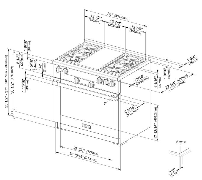
(x) = Toe-kick height adjustment  $4" - 5^{1/2}" (101.6 - 139.7 \text{mm})$
