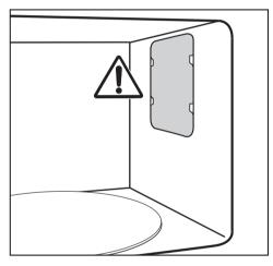
Do not remove the cover to the microwave outlet inside the oven, nor the film covering the inside of the door. Check the appliance for any damage.
