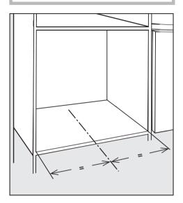
Draw a line inside the housing unit to mark the middle of the unit as illustrated.
