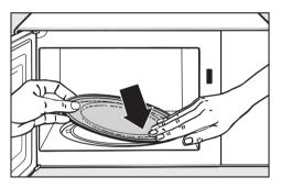
Remove the turntable, and wash in the dishwasher or by hand.
