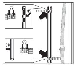
Secure the transit bars to the back of the washing machine. Make sure that holes ® are fitted over retainers A. The washing machine must not be moved without the transit bars in place.
