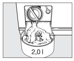
Unscrew the drain filter lid until water runs out.
