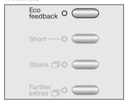
Press and hold the Eco feedback button after selecting the programme. The probable consumption levels will then be displayed by a bar chart.
