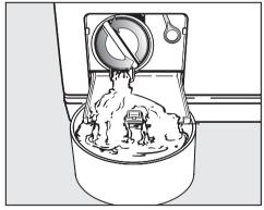
■ Slowly and carefully unscrew the drain filter to let the water out.
