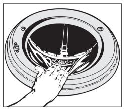
Check the folds in the door seal for any small articles e.g. buttons which might be lodged there.
