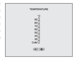
Use the I touch pads until the indicator light for the required temperature lights up.
