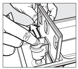
Remove the siphon from compartment <u>1</u><sup>®</sup>*I*.
