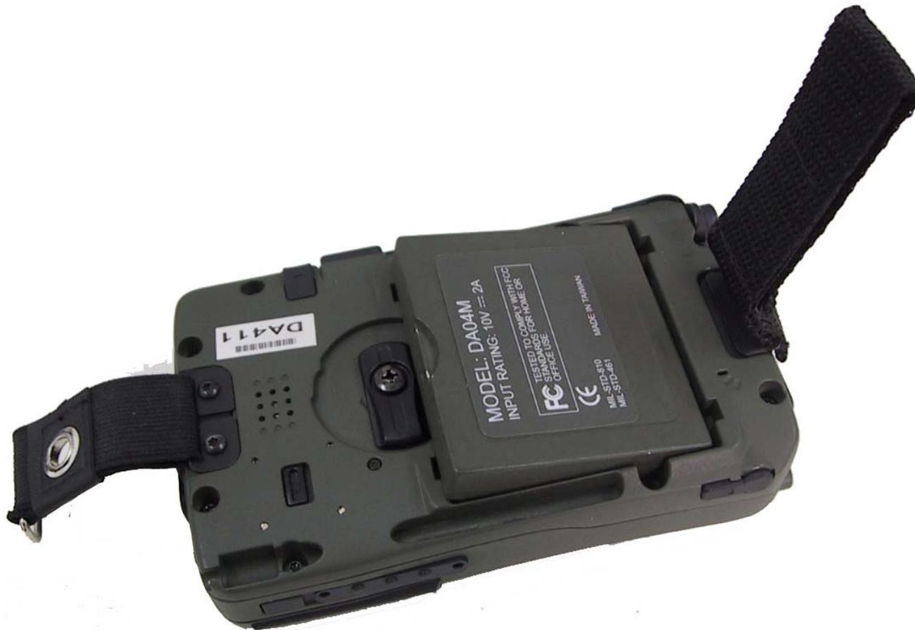
*Note: During battery swap the memory data is sustained by a small backup battery. Please swap battery within 1 minute to avoid data loss.*
