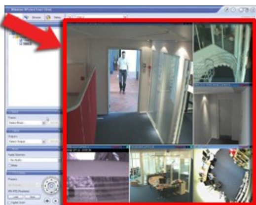
Example: Smart Client displaying view with six different cameras (view is highlighted in red frame)
