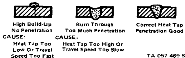
Figure 4-5. Cross Cut View of Various Welds
