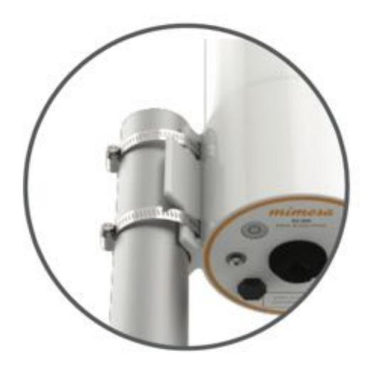
Using the included pole mount clamps, tightly attach the bracket to the top section of your mounting pole with a flathead screwdriver.
