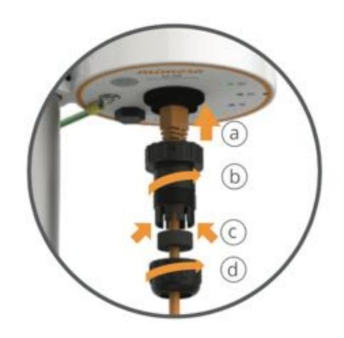
Use only shielded CAT 6 cabling and seal the system with the IP67 gland as shown.
