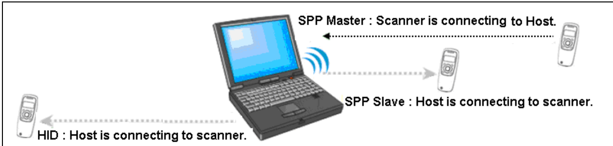
Figure 5-1. Diagram of Bluetooth functionalities
