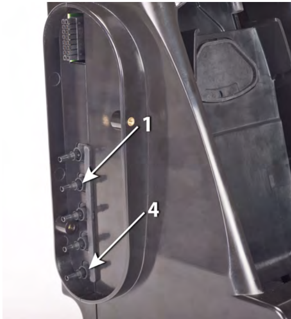
Fig. 17 Gas inlets on the Test Stand
