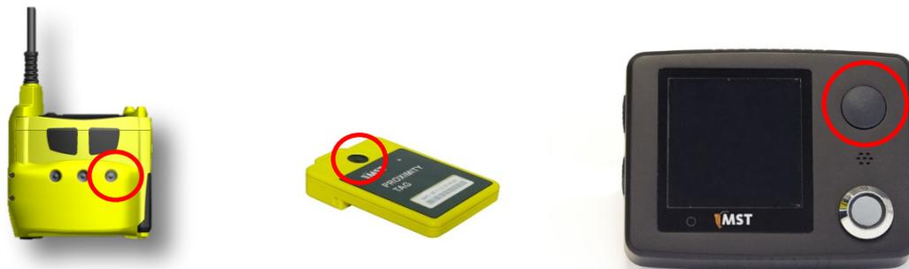
Pressing the suppression button on a personnel tag or ICCL embedded tag will suppress the vibration and the audible alarm; the LED will also stop flashing and illuminate permanently. Suppression of the alarms allows personnel to concentrate on taking corrective action. This suppression is only temporary and all the alarm behaviours will resume after a user configurable time span.
