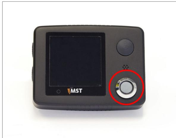
The iButton sensor is activated by inserting iButton fob supplied with the controller. When activated the system WiFi is enabled, which provides the user with access the system's configuration using standard web browsers.
