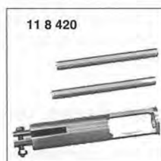
Valve removal and installation tool (BMW special tool 11 8 420)
