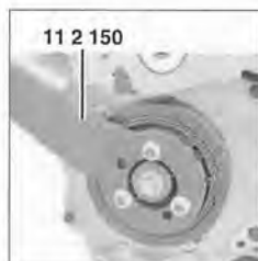
➤ Crankshaft vibration damper holder (Cooper) (BMW special tool 11 2 150)
