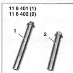
➤ Modular front end supports (BMW special tool 11 8 400)
