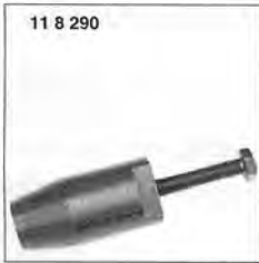
Extraction tool for rear main seal (BMW tool no. 11 8 290)
