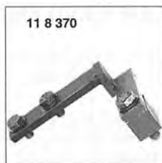
Engine block support tool (BMW special tool 11 8 370)
