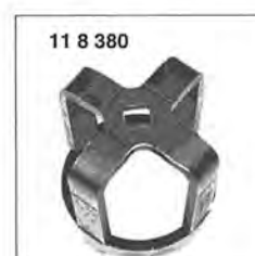
➤ Hydraulic engine mount removal and installation tool (BMW special tool 11 8 380)
