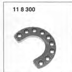
➤ Gear puller jig for crankshaft chain sprocket (BMW special tool 11 8 300)
