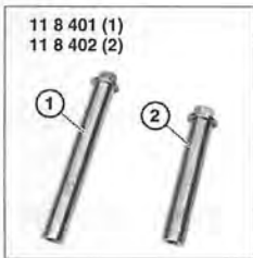
Modular front end extensions (BMW tool no. 11 8 400)
