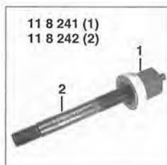
➤ Crankshaft vibration damper installation tools (BMW special tool 11 8 240)
