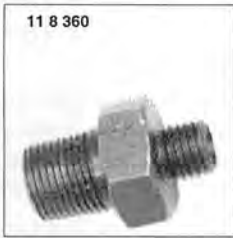
Oil pressure tool fitting (BMW tool no. 11 8 360)
