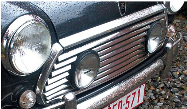
Part nr. 140.307 Stainless steel grill fitted with 6" spotlamps, for internal bonnet release
