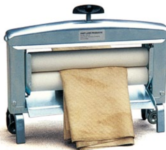
Part nr. 185.335 The professional wringer Heavy duty industrial quality wringer for chamois, towels etc. Specifications: Rustproof all steel frame, maintenance free rollers and bearings, adjustable pressure over the entire length of the rollers for uniform water removal. The complete wringer machine has two strong clamps for easy attaching.
