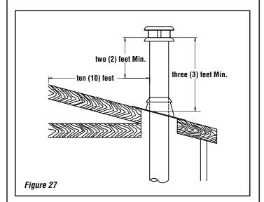
**Note:** 2" clearance to combustibles around chimney components required.
