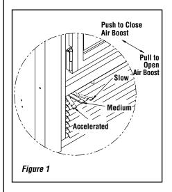
Use caution when firing with the combustion air control wide open. Only burn cord wood in this manner. Small dry pieces of softwood and construction scraps will burn very intensely using this method and may damage the firebox.
