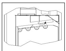
Figure 2a - Top Baffle Removal
