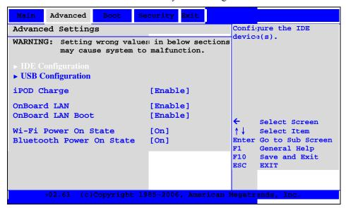
**IDE Configuration** sets the auto detection of the hard disk drive in your system.
