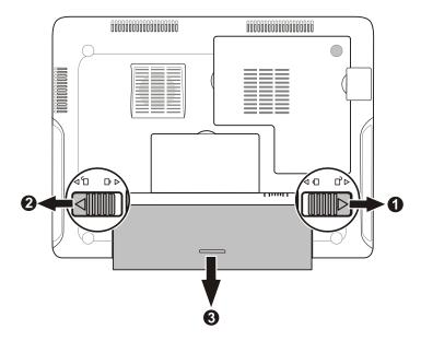
5. Fit another battery pack into place and slide the battery security lock to the lock (🗅) position.
