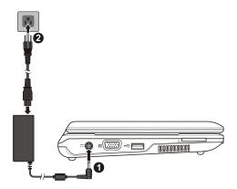
4. When the AC adapter is connected, power is being supplied from the electrical outlet to the AC adapter and onto your computer. Now, you are ready to turn on the computer.
