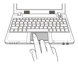
The touchpad consists of a rectangular pad and a left and right buttons. To use the touchpad, place your forefinger or thumb on the pad. The rectangular pad acts like a miniature duplicate of your display. As you slide your fingertip across the pad, the pointer (also called cursor) on the screen moves accordingly. When your finger reaches the edge of the pad, simply relocate yourself by lifting the finger and placing it on the other side of the pad.
