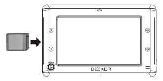
To remove a card, first make sure that no application is accessing the card, then slightly push the top edge of the card to release it and pull it out of the slot.
