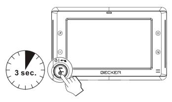
When you press the power button to turn off the unit, your device actually enters into a suspend state and the system stops operating.
