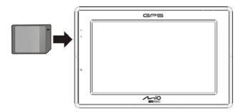
To remove a card, first make sure that no application is accessing the card, then slightly push the top edge of the card to release it and pull it out of the slot.
