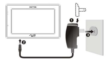
4. The charge indicator glows amber when charging is in progress. Do not disconnect your device from AC power until the battery is fully charged, the charge indicator will turn green. This will take a couple of hours.
