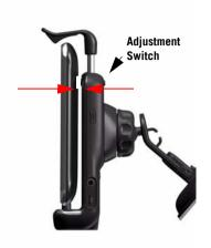
If there is a gap, you can slide the adjustment switch on the back to push out the adjustment block so that it rests against the back of your iPhone. (Please note, that if there is still a gap you will need to remove your iPhone. Then pull out the adjustment block, rotate it 180° and place it back in the cradle. This will increase the thickness of the adjustment block, providing for a snug fit.)
