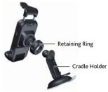
Press the unlock button and raise the retaining arm all the way to the top.
