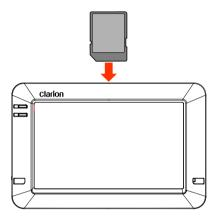
To remove a card, gently push the top edge of the card inwards to release it, and pull it out of the slot.
