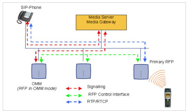
To establish a call between two PPs, the same IP streams must be established like in the scenario before, except the IP phone is not involved. The following figure illustrates this scenario.
