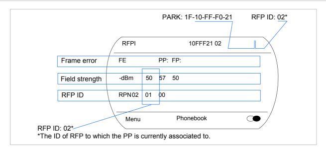
In this example the PP is currently connected to the RFP with the number 02. The RFPs 01 and 00 are also visible. The number "10FFF221 02" on the upper right side refers to the PARK (Example 1F-10-F2-21) of the SIP–DECT system and to the RFP to which the phone is currently connected to.
