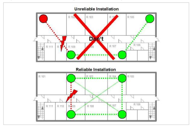
The sync-over-air solution is very reliable because all existing redundant paths are used for synchronization. Thus, hardware tolerances have only very little influence. No RFP has a key position.
