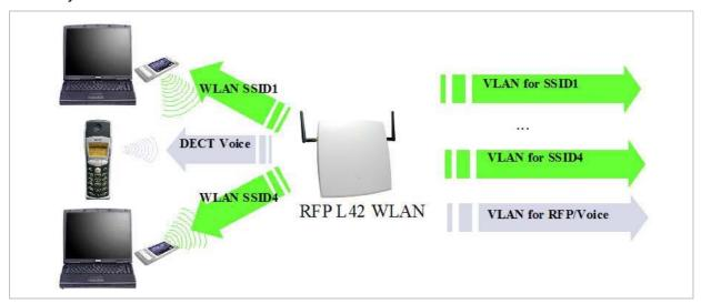
The access point can be assigned to a VLAN that conforms to 802.1q. All the data that is received from and that is to be forwarded to the WLAN clients is then carried by the configured VLAN. All other data, such as VoIP packets, configuration data or authentication data (Radius), is given the VLAN tag configured for the RFP. The switch port of the network component to which the access point is connected must be configured as a trunk port.
