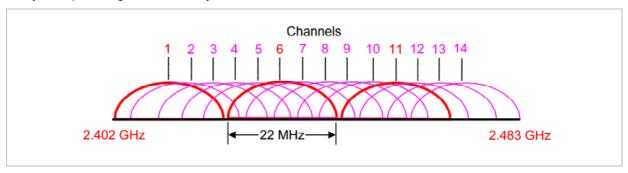
When planning the radio coverage for a two-dimensional area, please bear in mind that the distance between any two base stations operating on the same frequency must be at least twice their range. The range can be adjusted by lowering the output power level.
