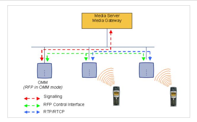
A call from one PP to another that resides on the same RFP will loop back within the RFP if no media gateway is involved. So the call will not pass through to the Local Area Network (LAN). Although the voice packets will not impact LAN traffic, signal packets will.
